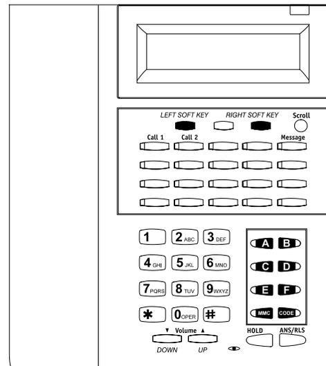
This diagram illustrates the keys on a **iDCS 8 BUTTON** keyset that have special functions during programming. When required, these keys will be referred to by the names described in the diagram.
